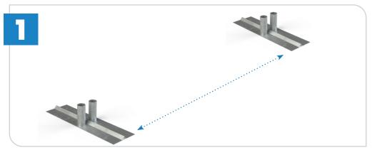
Place the fence foot on the ground and walk out the length of the first barrier, then place the second foot on the ground. Set down each barrier alongside your desired fence line.
